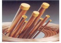
Standard copper tubing is for water, plumbing and house vacuum applications. For the delivery of flammable gases, inert gases, and compressed air, use Type K and Type L copper tubing (Generally Size: NPS 3/8"). Use 300 psig minimum pressure rating downstream from a pressure regulator.
