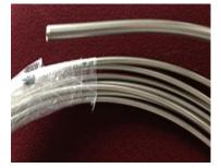
Stainless steel tubing, grade 316L, is required for the delivery of hydrogen and toxic gases to research equipment. Use nominal size is ¼" ID with minimum pressure rating 300psig at the range of applied laboratory temperatures. Connect with Swagelok VCR fittings or similar. Leak check before use.
