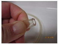
Softwall tubing and hoses are generally for inert gases and low pressure water. Do not use in "out-of-sight" applications where the hose is buried, encased or submerged. Use rigid tubing in these applications.
