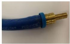
At room temperature, acceptable for use with inert gases (some lighter gases may permeate the hose), compressed air (safety factor 4:1), oxidizers, house vacuum systems. Push on hoses can be rated to 350psig when used with the manufacture's barb connector. Nominal size of 3/8" and smaller diameters require no special tools for assembly.
