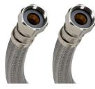
Use for permanent connections to building water and process cooling. Labs are to use stainless steel braided hose when connected to process chilled water rated for 175 psi. Connections are to be threaded.
